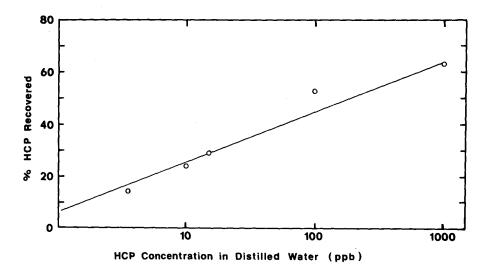
Figure 2. Efficiencies of Water Extraction Procedure (Least squares line of best fit).
